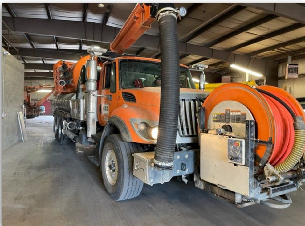
A VECTOR JET TRUCK IS SEEN. THE TRUCK IS USED TO CLEAN OUT THE STORM SEWER COLLECTION SYSTEM.
